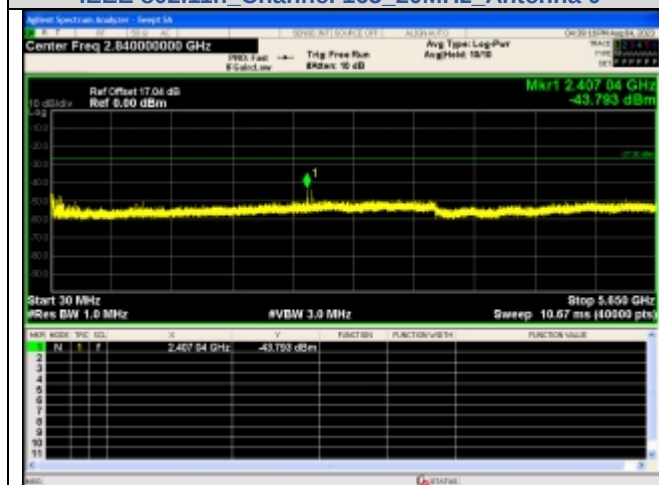
Spurious Emission:30.0~5650 MHz IEEE 802.11n Channel 151 40MHz Antenna 0
