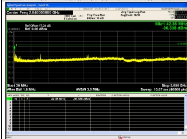
Spurious Emission:30.0~5650 MHz IEEE 802.11ac Channel 149 20MHz Antenna 0
