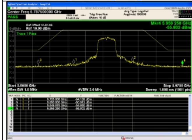
Out Of Band Emission IEEE 802.11n Channel 159 40MHz Antenna 0
