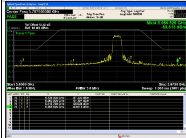
Out Of Band Emission IEEE 802.11n Channel 165 20MHz Antenna 0
