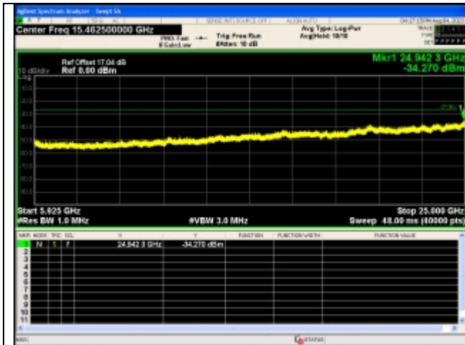
Spurious Emission:5925~25000.0 MHz IEEE 802.11n Channel 149 20MHz Antenna 0
