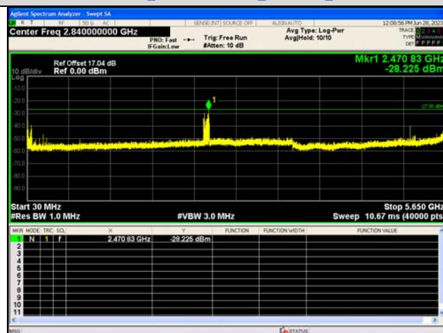
Spurious Emission:30.0~5650 MHz IEEE 802.11ac_Channel 155_80MHz_Antenna 0
