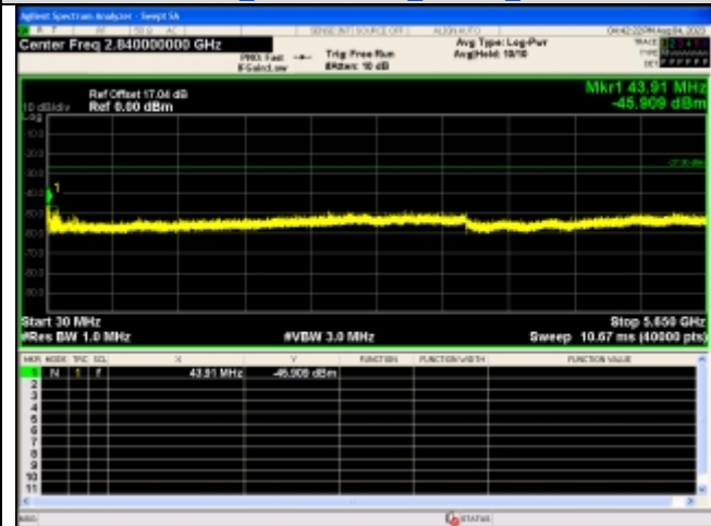
Spurious Emission:30.0~5650 MHz IEEE 802.11n Channel 159 40MHz Antenna 0
