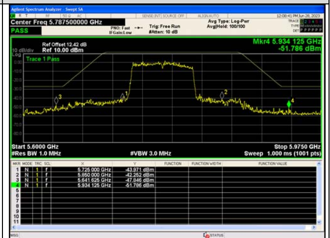
Out Of Band Emission IEEE 802.11ac_Channel 155_80MHz_Antenna 0
