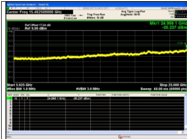
Spurious Emission:5925~25000.0 MHz IEEE 802.11n Channel 159 40MHz Antenna 0
