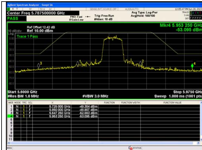
Out Of Band Emission IEEE 802.11ac_Channel 159_40MHz_Antenna 0
