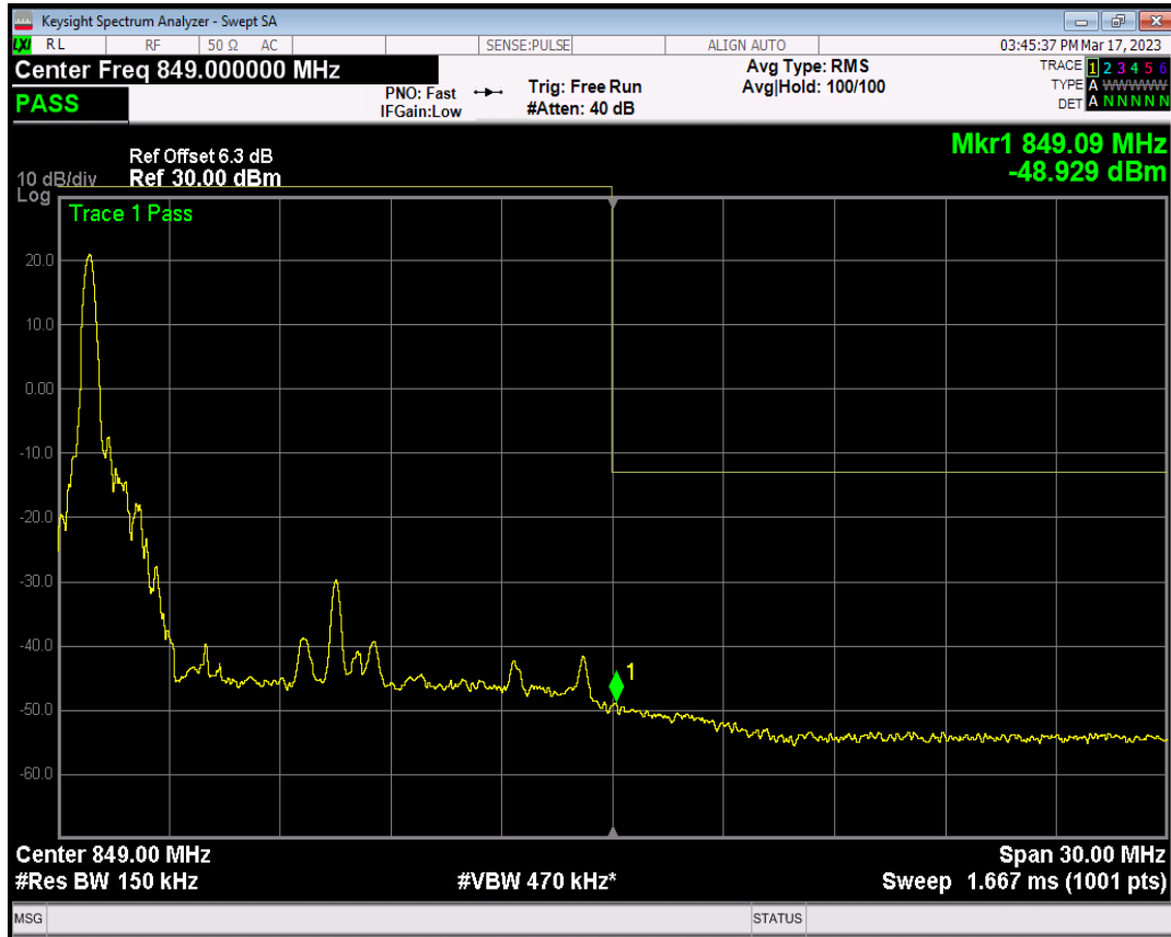
Band26(824-849) QAM16 BW=15MHz Channel=26965 RB Size=1 Position=#Max
