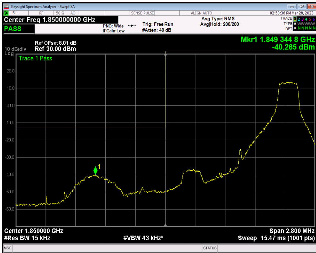
Band2 QPSK BW=1.4MHz Channel=18607 RB Size=6 Position=#0
