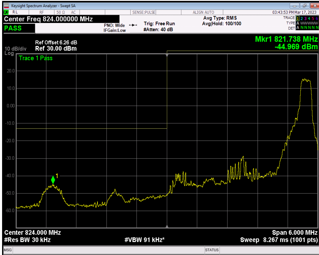
Band26(824-849) QAM16 BW=3MHz Channel=26805 RB Size=15 Position=#0
