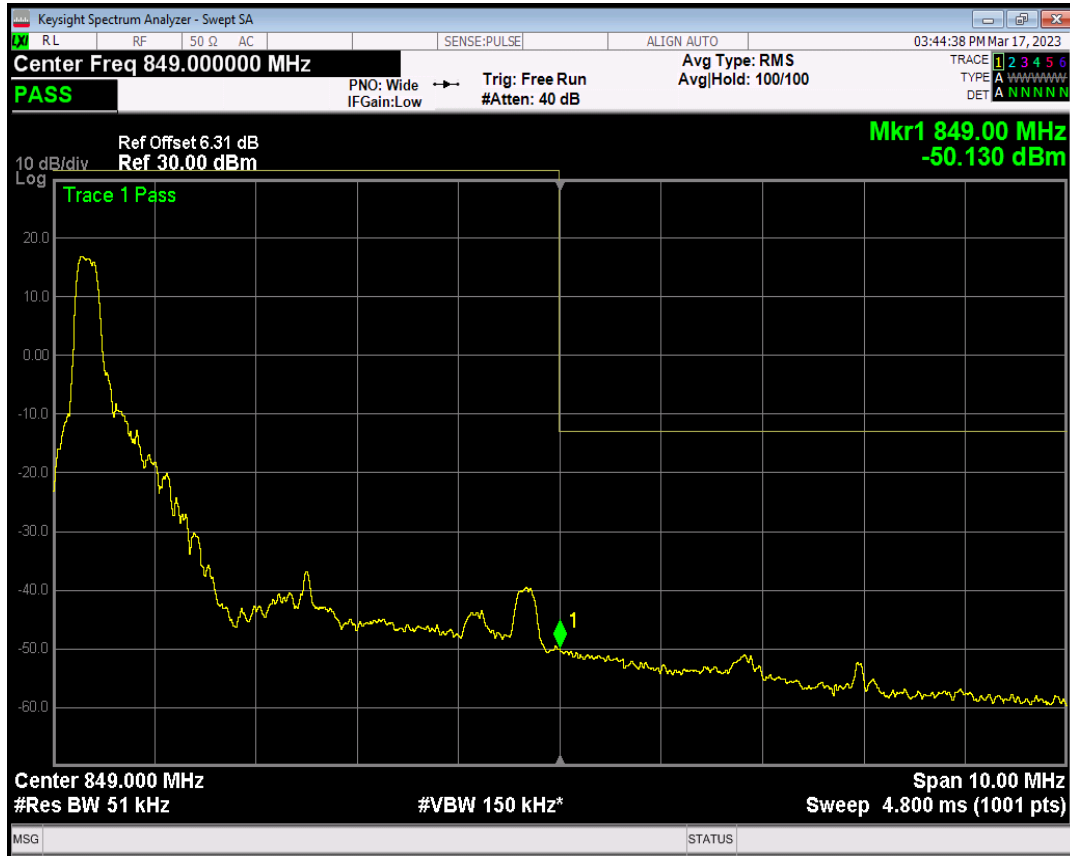
Band26(824-849) QAM16 BW=5MHz Channel=27015 RB Size=1 Position=#Max
