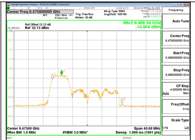
LOW CHANNEL Antenna 3
