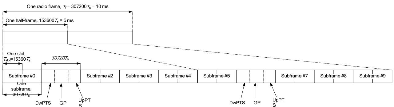
The period of the GAP is configured by base station from 66.7us to 667us, see bellows chart: 'GP' is the GAP, and one symbols is 66.7us.
