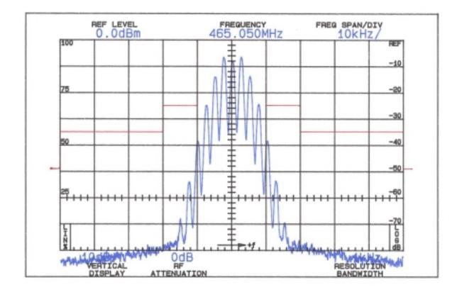
On any frequency more than 50% up to and including 100% of the authorized bandwidth, 20 kHz (10-20 kHz)
