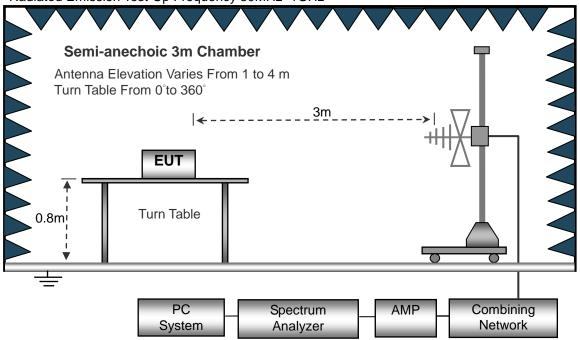
(C) Radiated Emission Test-Up Frequency Above 1GHz
