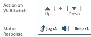
\*The operation is only valid when there are no limits. If the motor has already set the upper and lower limit, then you can only switch direction by pressing “P1” button (about 10 sec) on the motor head until motor jog x3 and beep x3.
