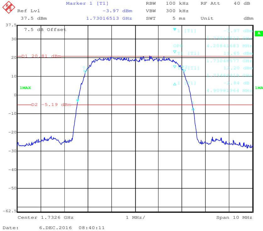
26 dB Emissions Bandwidth & 99% Occupied Bandwidth for HSDPA (16QAM) Mode
