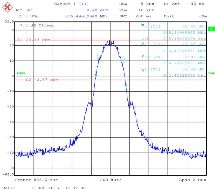
**26 dB Emissions & 99% Occupied Bandwidth for RMC (BPSK) Mode**
