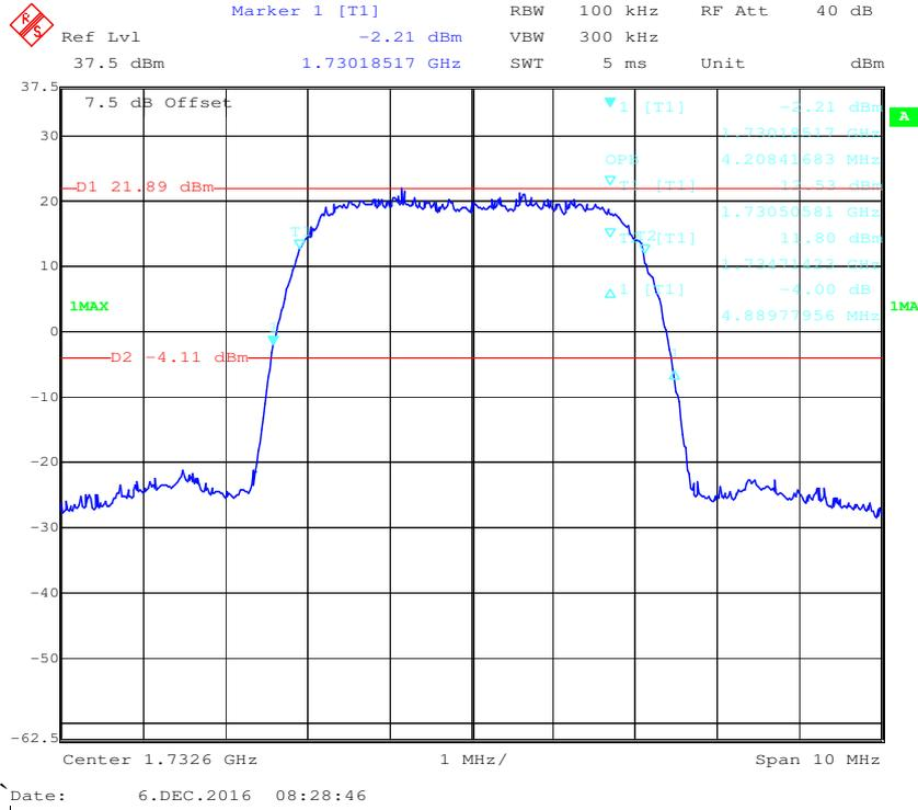
**26 dB Emissions Bandwidth & 99% Occupied Bandwidth for HSUPA (BPSK) Mode**
