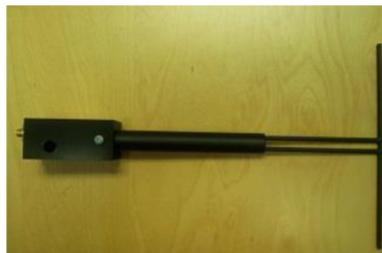
**Figure 1 – MVG COMOSAR Validation Dipole**
