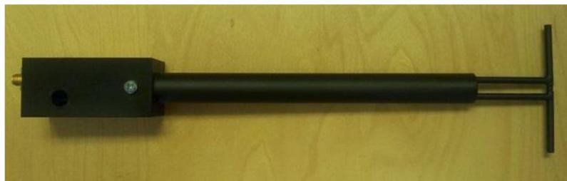
**Figure 1 – MVG COMOSAR Validation Dipole**
