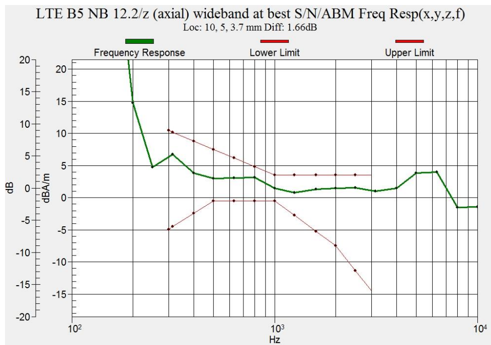
Figure B.6 Frequency Response of LTE Band 5
