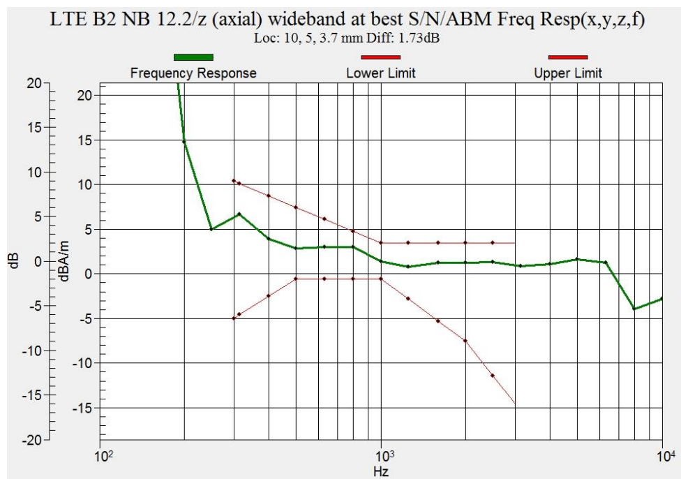
Figure B.4 Frequency Response of LTE Band 2
