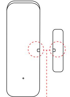
The alignment marks must be close together as possible. **Must be ≤15mm**
