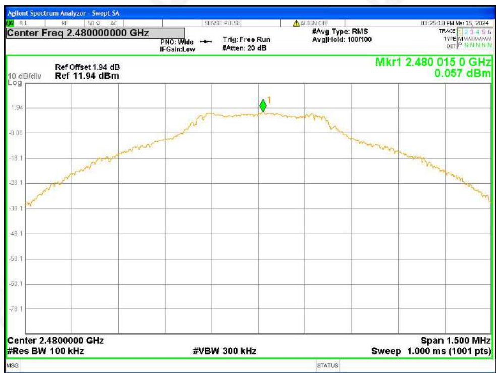
Tx. Spurious NVNT 1-DH5 2480MHz Ant1 Ref
