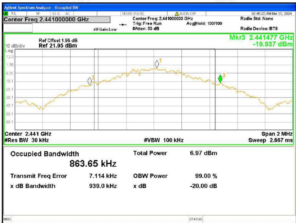
-20dB Bandwidth NVNT 1-DH5 2441MHz Ant1
