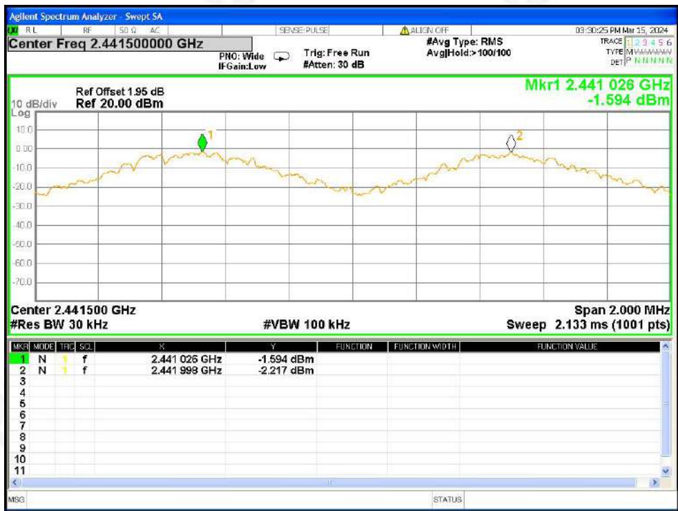
CFS NVNT 1-DH5 2441MHz Ant1
