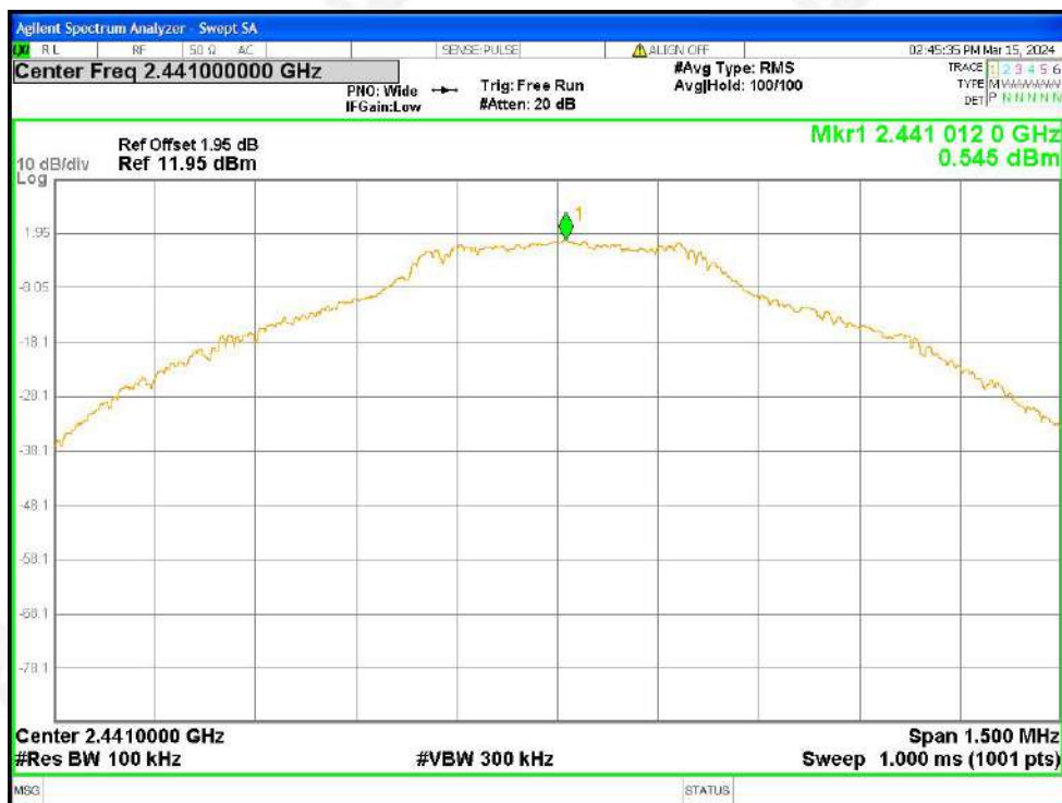
Tx. Spurious NVNT 1-DH5 2441MHz Ant1 Ref
