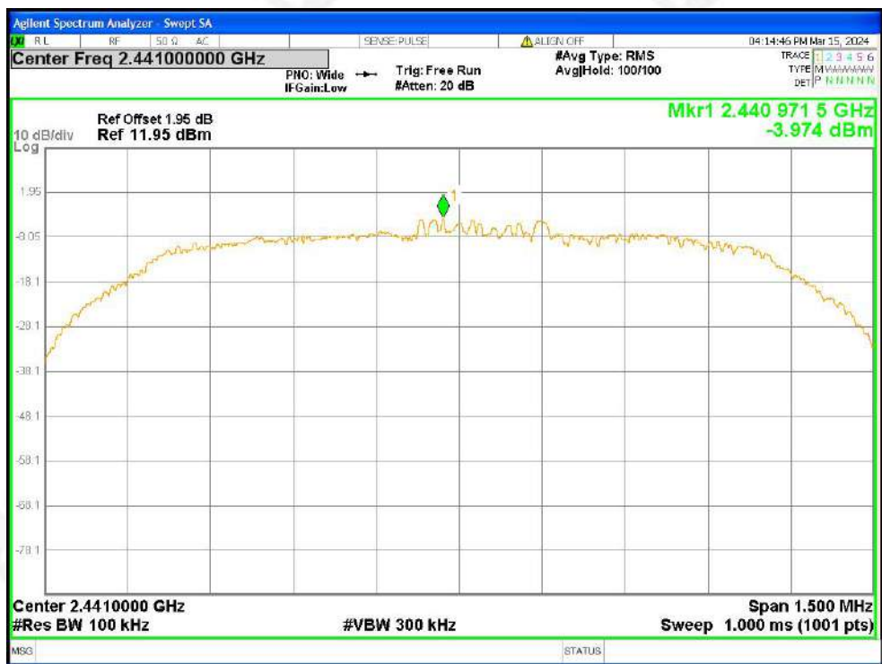
Tx. Spurious NVNT 2-DH5 2441MHz Ant1 Ref
