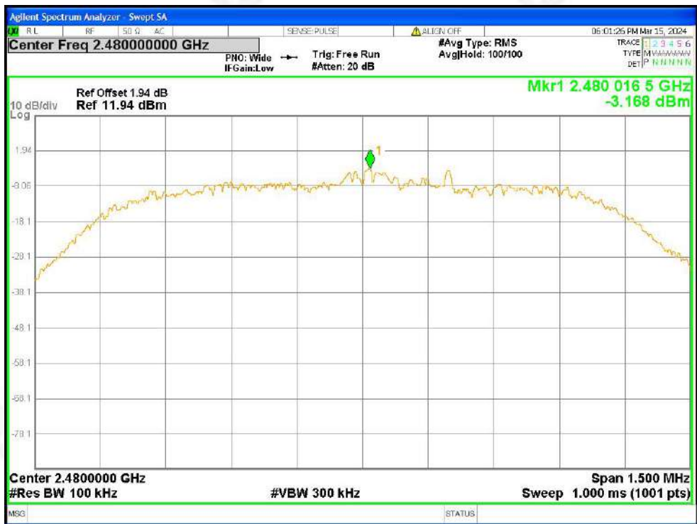
Tx. Spurious NVNT 3-DH5 2480MHz Ant1 Ref
