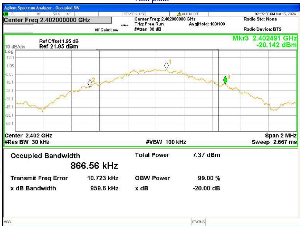
-20dB Bandwidth NVNT 1-DH5 2402MHz Ant1
