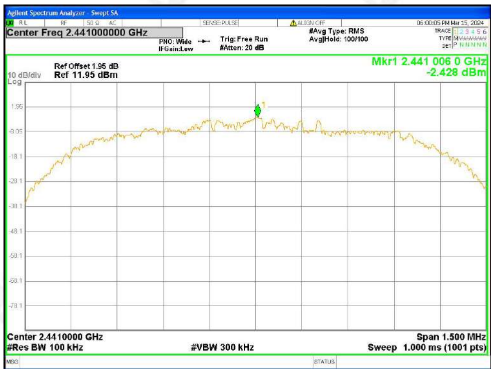
Tx. Spurious NVNT 3-DH5 2441MHz Ant1 Ref
