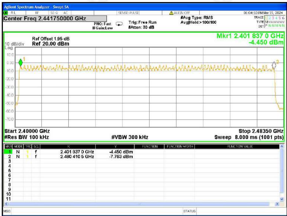
Hopping No. NVNT 3-DH5 2402MHz Ant1
