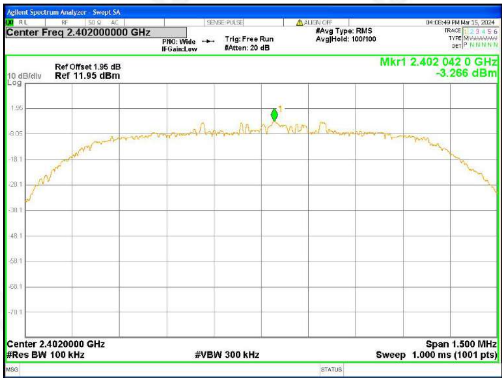
Tx. Spurious NVNT 2-DH5 2402MHz Ant1 Ref
