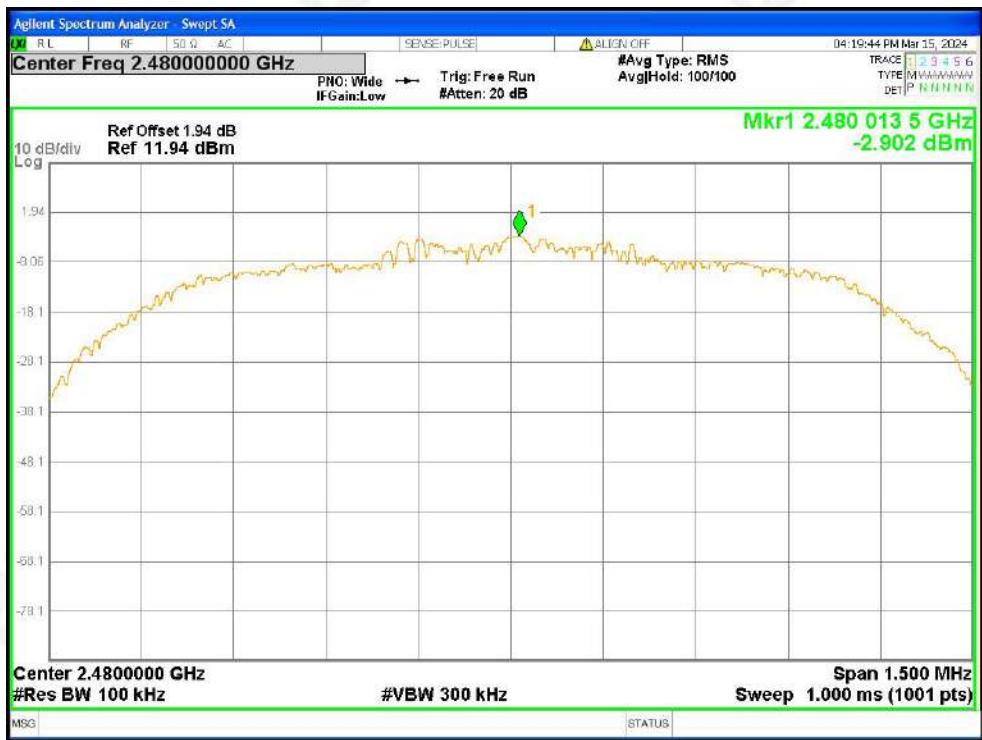
Tx. Spurious NVNT 2-DH5 2480MHz Ant1 Ref
