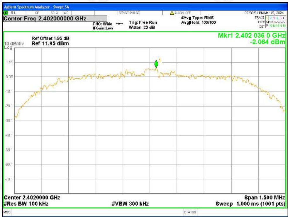
Tx. Spurious NVNT 3-DH5 2402MHz Ant1 Ref
