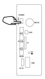
Slide the power switch to the ON position to power ON the speaker . After powering ON, the speaker will automatically go into Bluetooth pairing mode.
