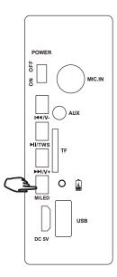
Press and hold the Light button to switch the lighting mode.
