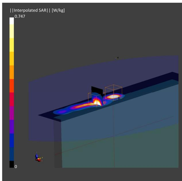
**5. LTE Band 12, QPSK - 10MHz, CH23130, Antenna Ant 5, Back face**
