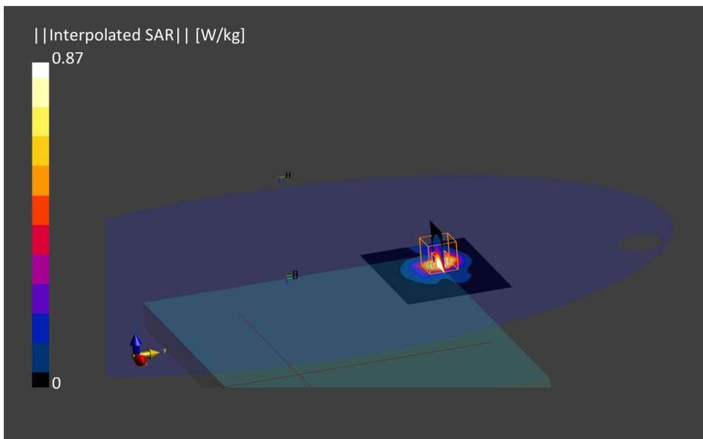
**11. LTE Band 41, QPSK - 20MHz, CH40620, Antenna Ant 8, Top edge**
