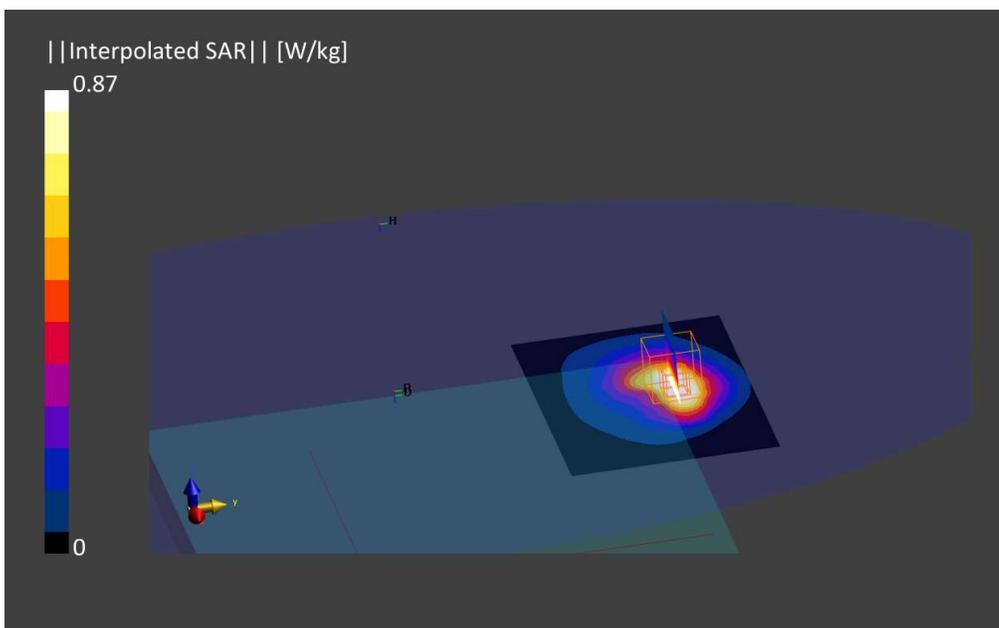
**6. LTE Band 13, QPSK - 10MHz, CH23230, Antenna Ant 5, Back face**
