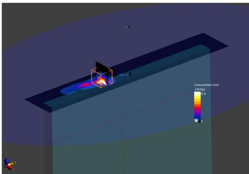
**13. LTE Band 66, QPSK - 20MHz, CH132572, Antenna Ant 5, Back Face**
