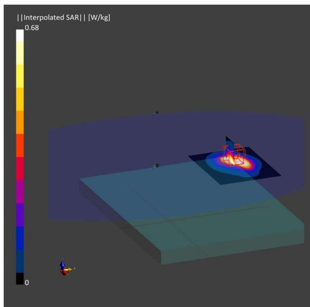
**4. LTE Band 7, QPSK - 20MHz, CH21350, Antenna Ant 8, Top Edge**
