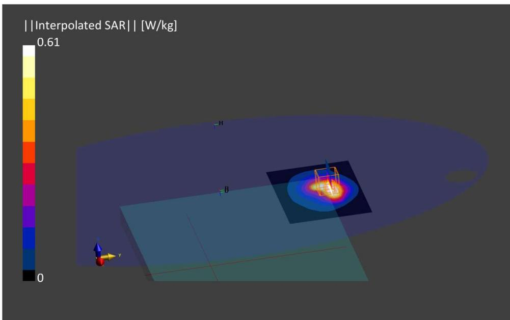
**7. LTE Band 14, QPSK - 10MHz, CH23330, Antenna Ant 5, Back face**
