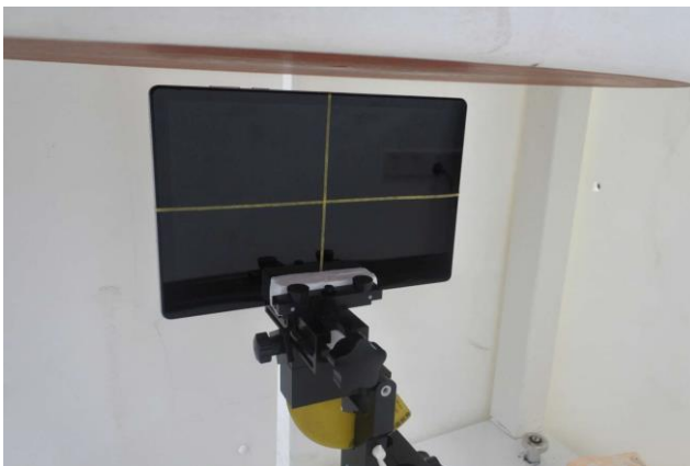
Edge 2 of EUT with Phantom 16 mm Gap (Sensor off)
