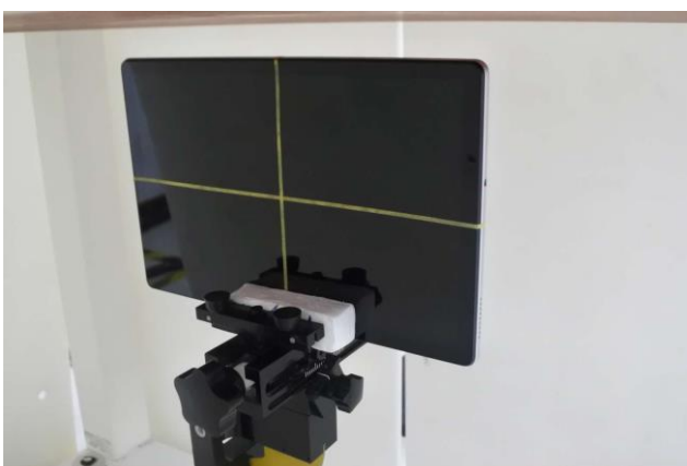
Edge 4 of EUT with Phantom 22 mm Gap (Sensor off)
