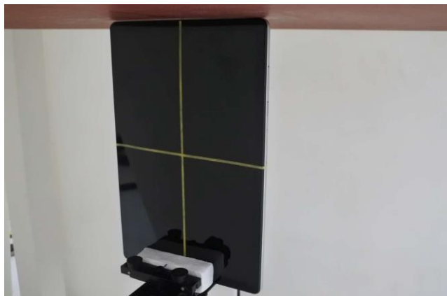
Edge 1 of EUT with Phantom 0 mm Gap
