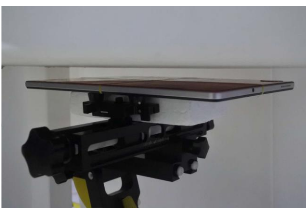
Bottom Face of EUT with Phantom 15 mm Gap (Sensor off)
