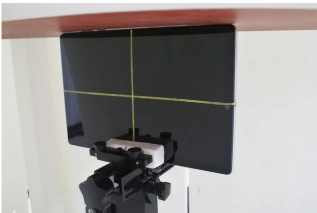
Edge 2 of EUT with Phantom 0 mm Gap
