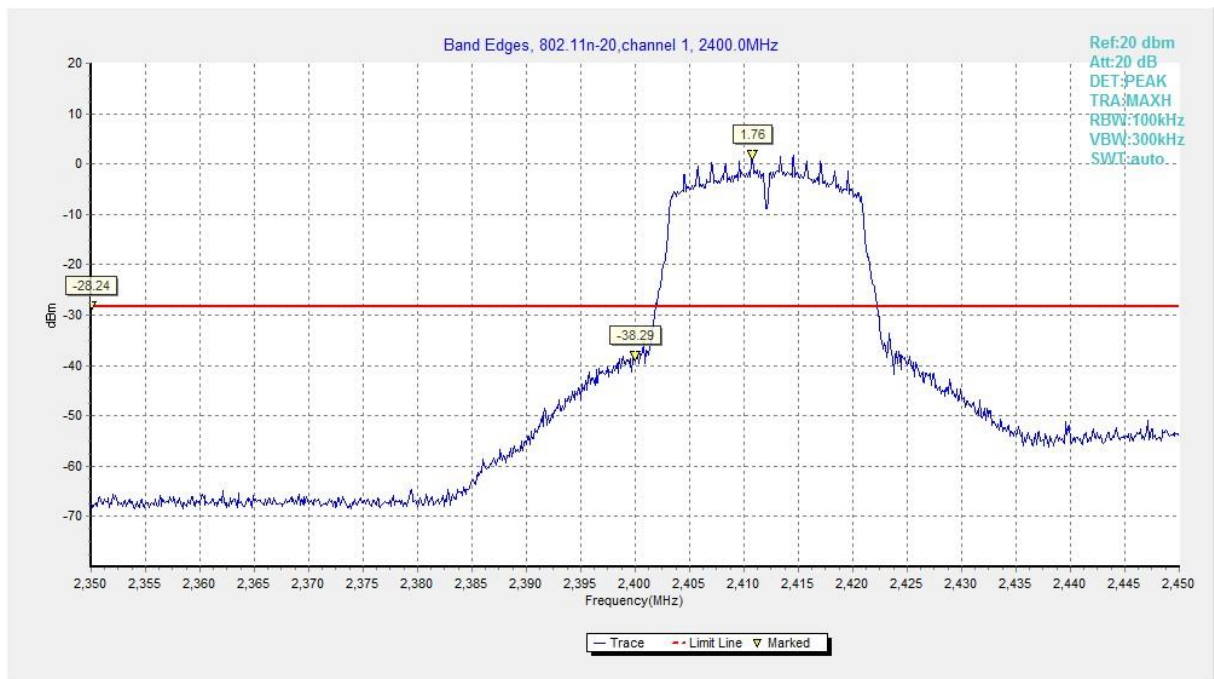
Fig.23 Band Edges (802.11n-HT20, CH 1)
