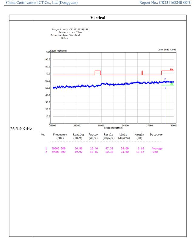
Test plots for Band Edge Measurements (Radiated)
