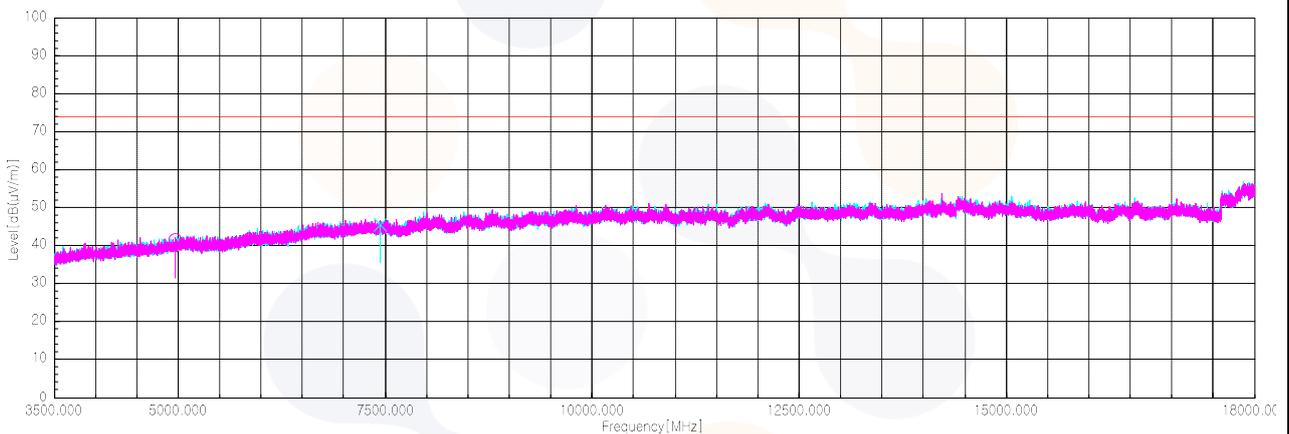
**Test results (Above 18 GHz) – Worst case: 2 Mbits/s(37 Bytes) 2 480 MHz**
