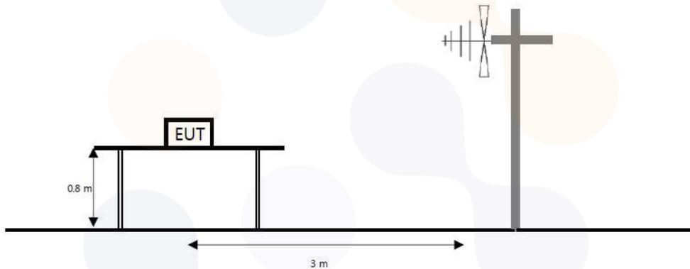
The diagram below shows the test setup that is utilized to make the measurements for emission from 1 GHz to the tenth harmonic of the highest fundamental frequency or to 40 GHz emissions, whichever is lower.
