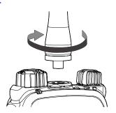
To remove the antenna, rotate it counter-clockwise.
