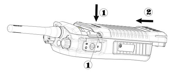
2. Open the battery latch and hold it down until the metal lock goes into the battery housing completely.
