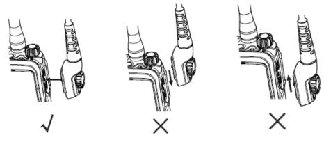
Step 3 Tighten the screw on the connector.
