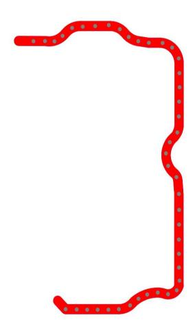
Remote control antenna specification Antenna size: 433M, antenna, material: Copper The antenna is whip with a width of 1.2mm a thickness of 1 oz and a total straightening length of 66mm Antenna Gain: OdBi
