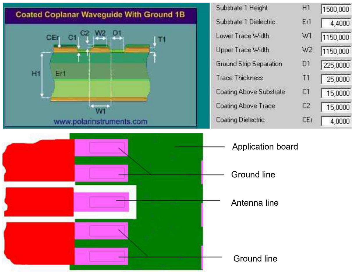
Figure 43: Micro-Stripline on 1.5mm Standard FR4 PCB - example 2
