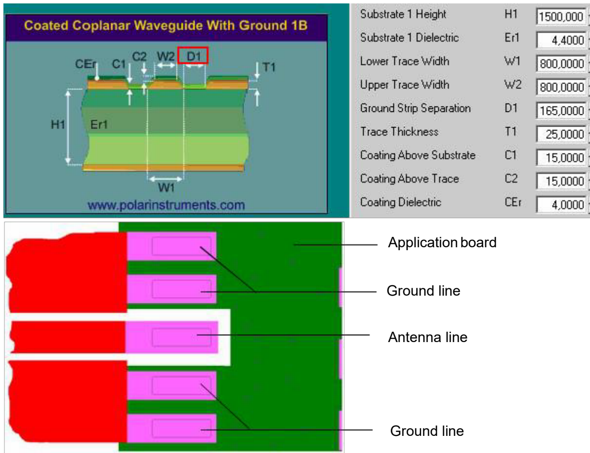
Figure 42: Micro-Stripline on 1.5mm Standard FR4 PCB - example 1
