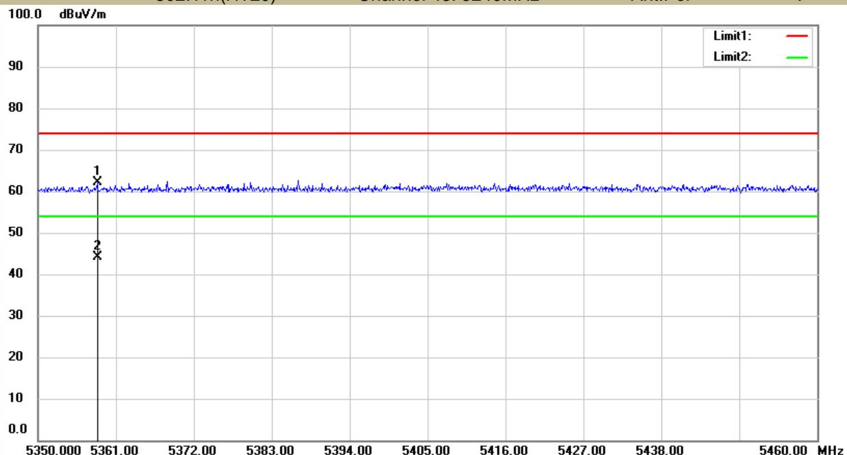
■ For Undesirable radiated Spurious Emission in U-NII -2A
