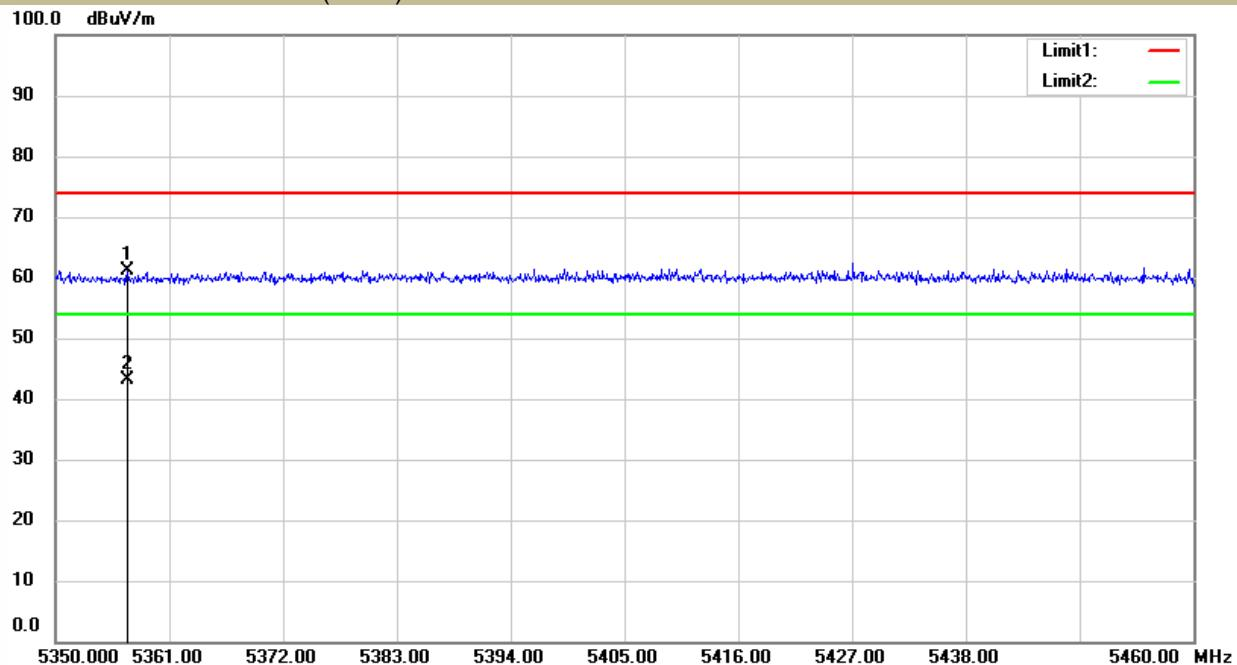
■ For Undesirable radiated Spurious Emission in U-NII -2C
