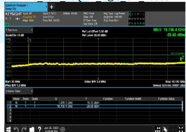
B25 15M 16QAM 1@0 CH 26365
