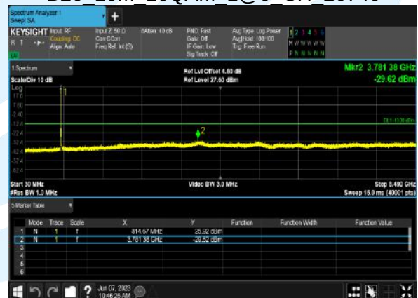
B26 10M 16QAM 1@0 CH 26740
