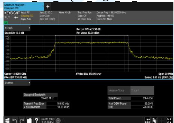
B25 15M 16QAM 75@0 CH 26365
