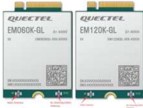
Figure 26: Antenna Connectors on the EM060K-GL and EM120K-GL
