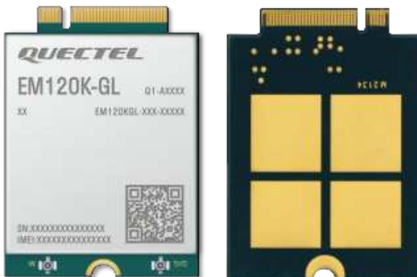
Figure 35: EM120K-GL Top and Bottom Views
