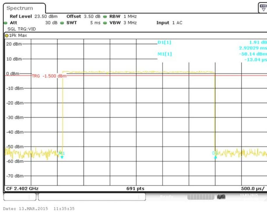
**Pulse time, Middle Channel, 2DH5**
