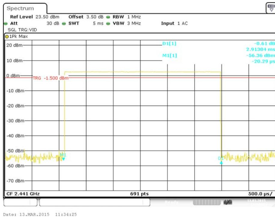
**Pulse time, High Channel, DH5**
