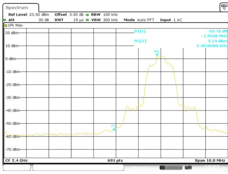
**EDR ( $\pi/4$ -DQPSK): Band Edge-Right Side**
