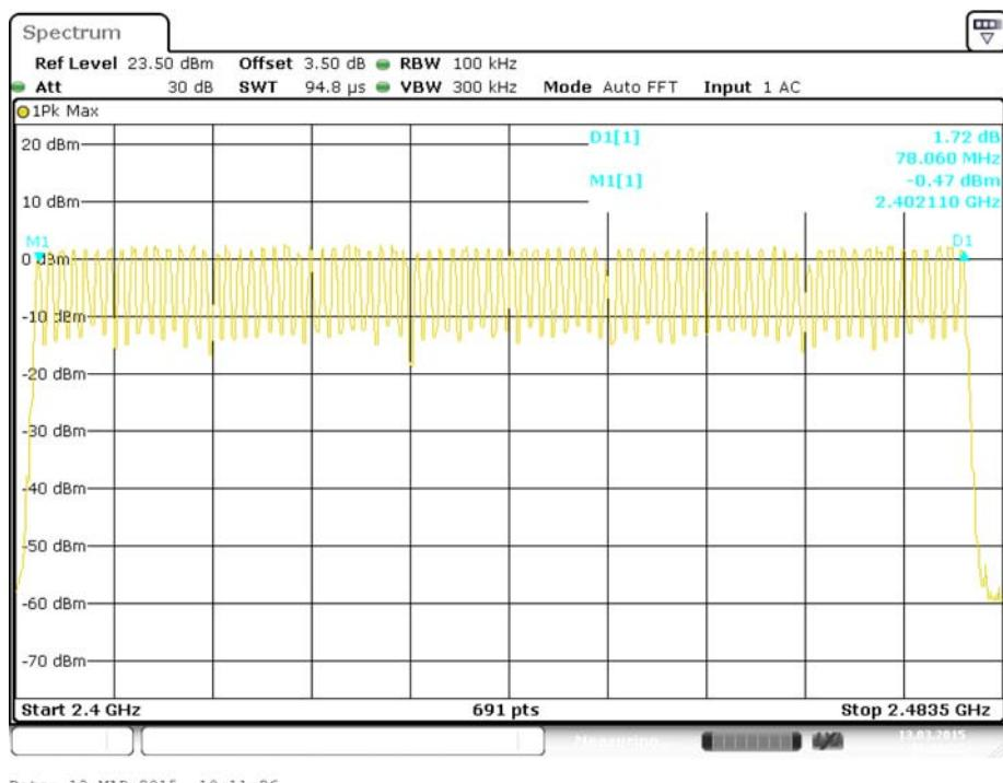
**EDR ( $\pi/4$ -DQPSK): Number of Hopping Channels**
