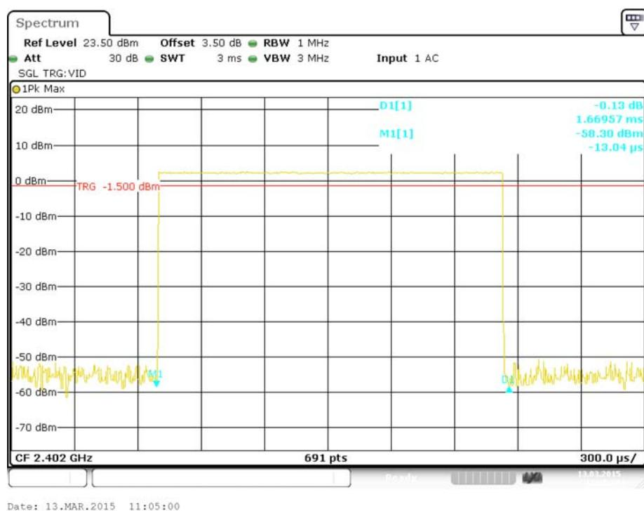
**Pulse time, Middle Channel, DH3**
