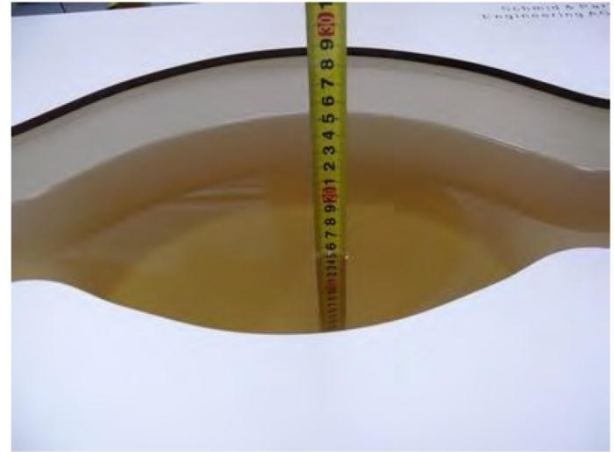
Liquid depth in the body phantom (835MHz)
