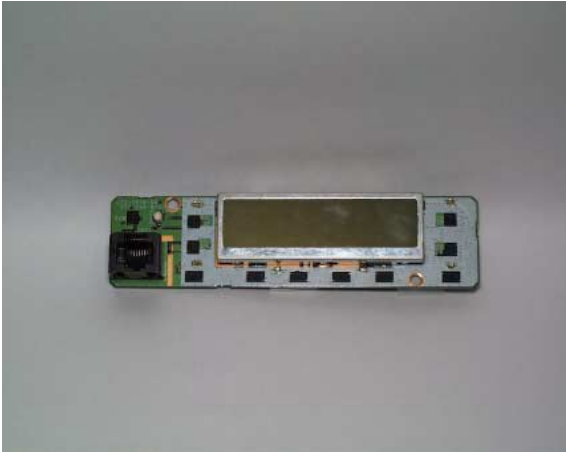
PCB Display 128ch Front View Model name:TK-860GK2/TK-862GK2 FCC ID:ALH29383120
