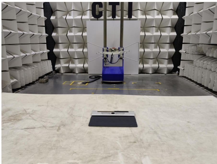
Radiated spurious emission Test Setup-2(Below 1GHz)
