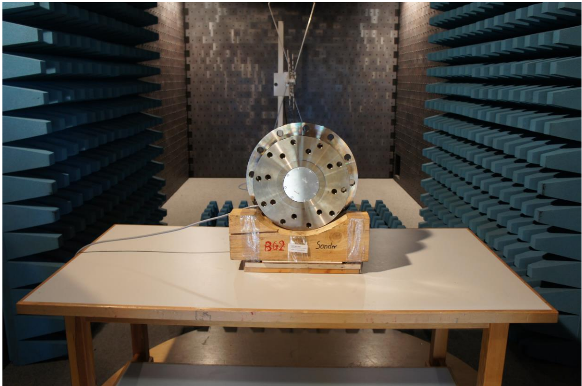
Picture 3: Test setup radiated emission test 30MHz - 1GHz, CDC
