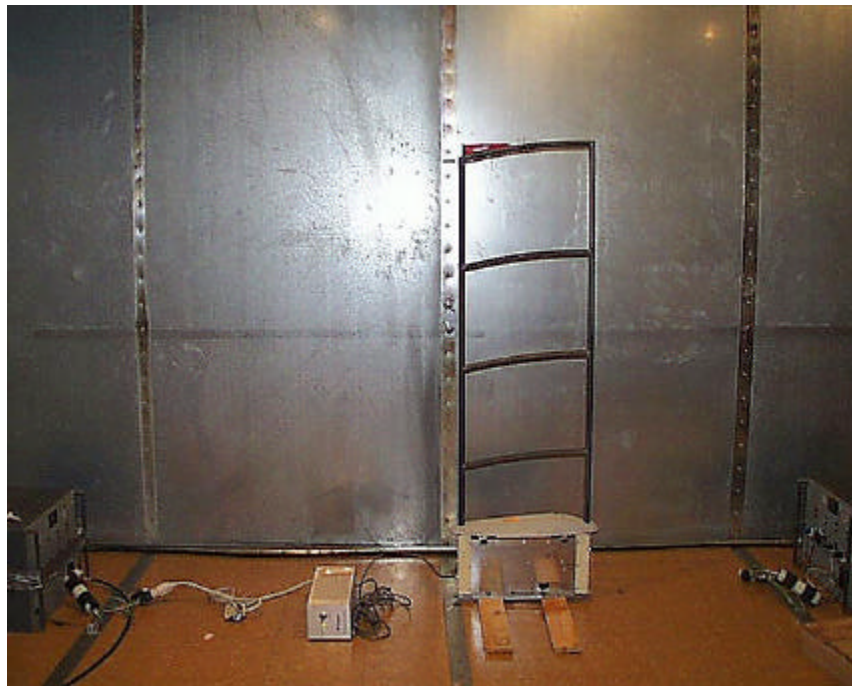
Photo 7 – Strata GX Conducted Emissions Test Setup
