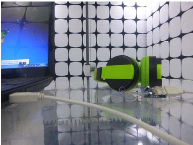
Radiated Spurious Emissions Test Above 1GHz
