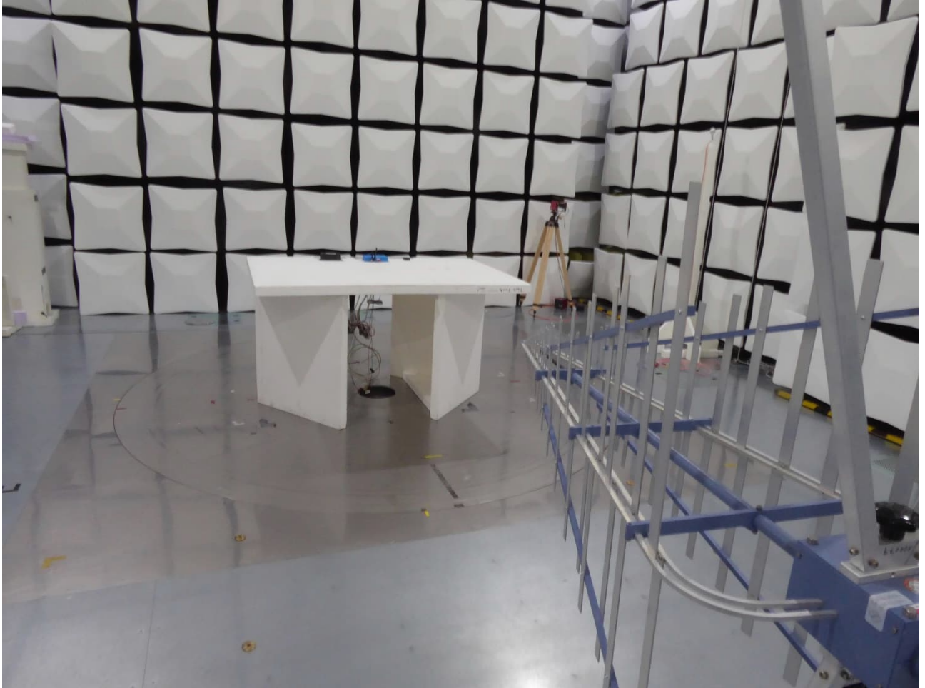
Test setup semi anechoic chamber M276, 30 MHz – 1 GHz
