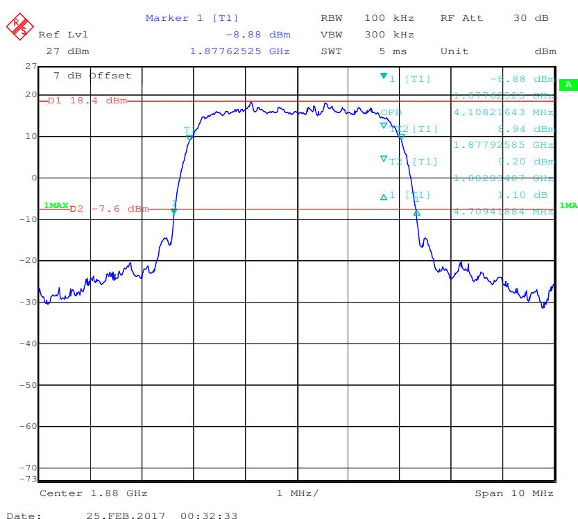
**99% Occupied Bandwidth & 26 dB Emissions Bandwidth for HSUPA (BPSK) Mode**
