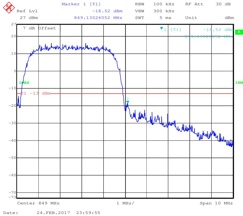
**PCS Band, Left Band Edge for GSM (GMSK) Mode**
