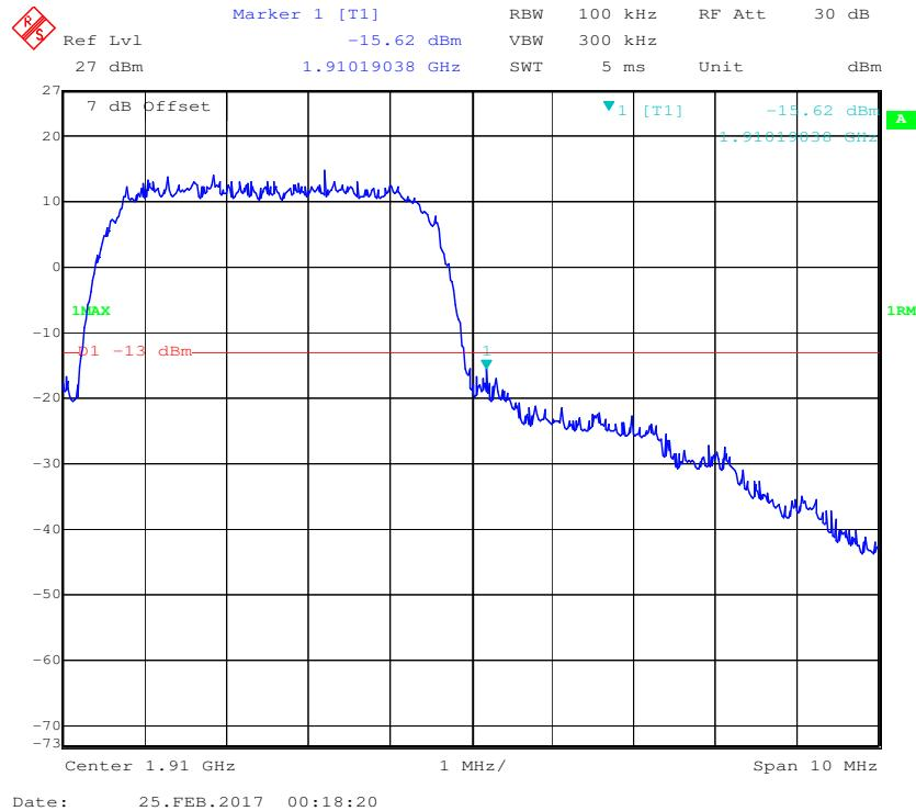
**PCS Band, Left Band Edge for HSUPA (BPSK) Mode**
