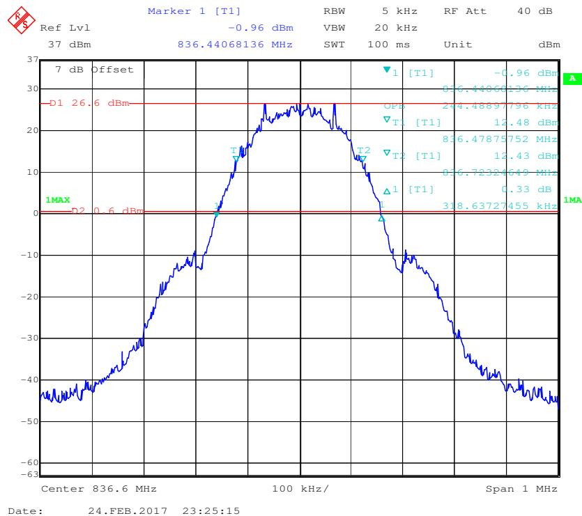
**99% Occupied Bandwidth & 26 dB Emissions Bandwidth for RMC (BPSK) Mode**
