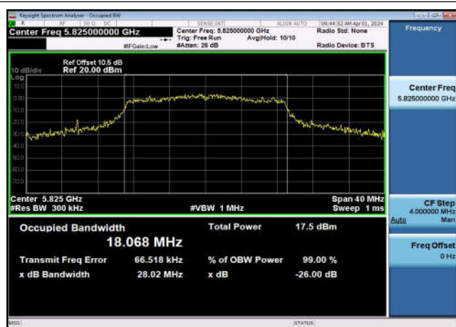
U-NII-3 99% & 26dB Bandwidth-802.11n(20MHz),5825MHz,Ant1
