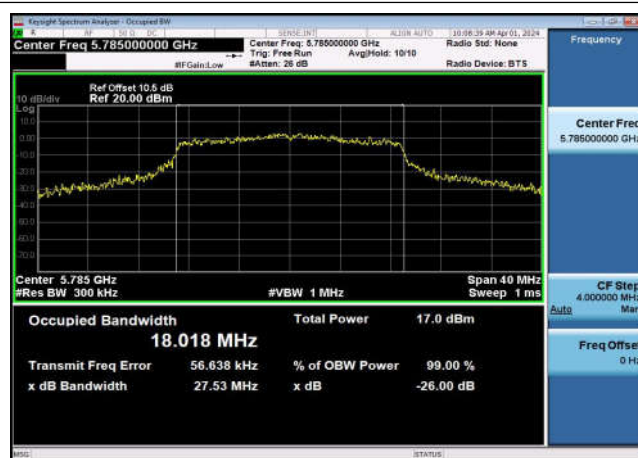
U-NII-3 99% & 26dB Bandwidth-802.11ac(20MHz) ,5785MHz,Ant1
