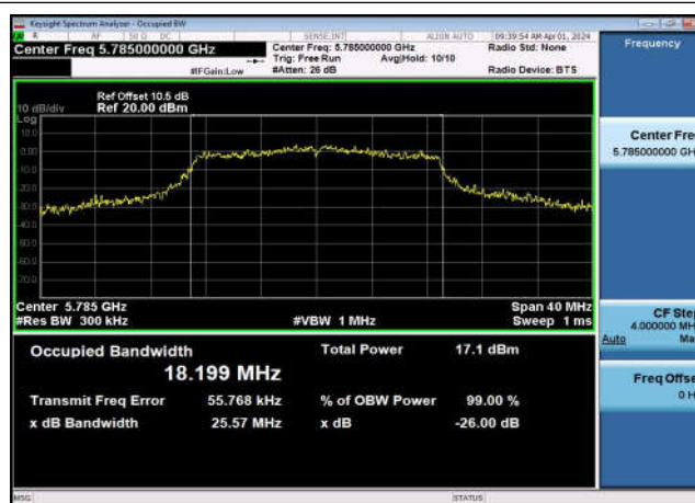
U-NII-3 99% & 26dB Bandwidth-802.11n(40MHz),5755MHz,Ant1
