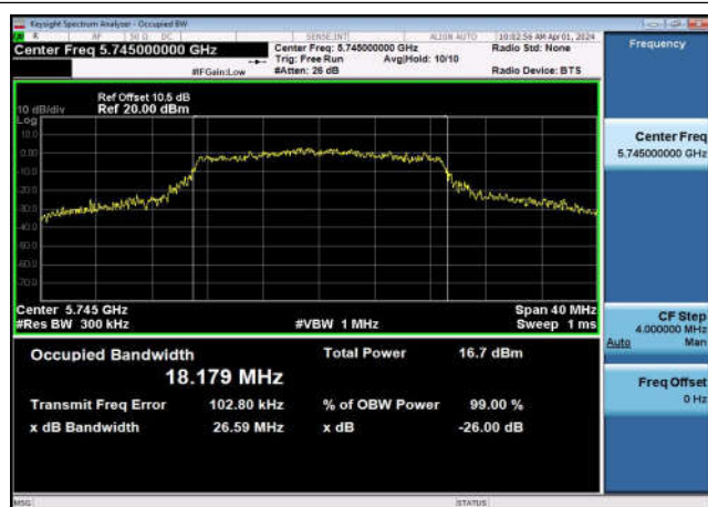
U-NII-3 99% & 26dB Bandwidth-802.11ac(20MHz) ,5745MHz,Ant1
