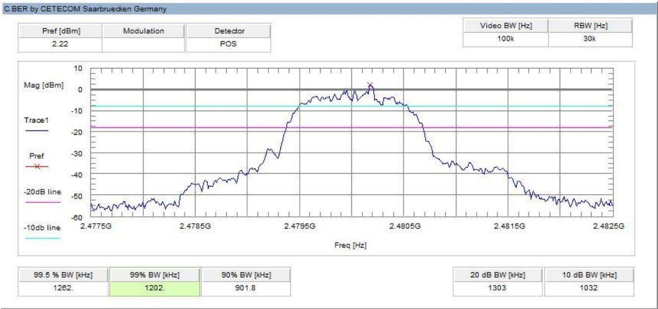
Plot 9: highest channel – 2480 MHz, 8 DPSK modulation
