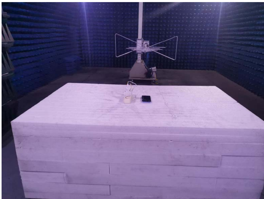
Photo of Radiated Emission Measurement (Above 1G)
