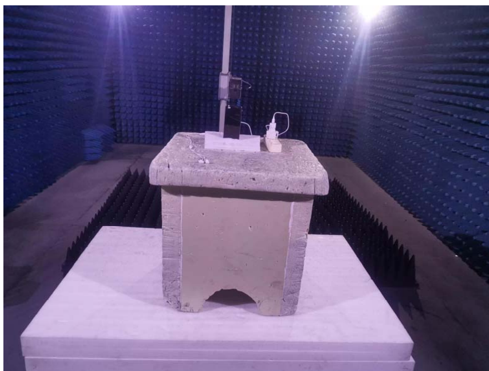
Photo of Radiated Emission Measurement (Above 1G)
