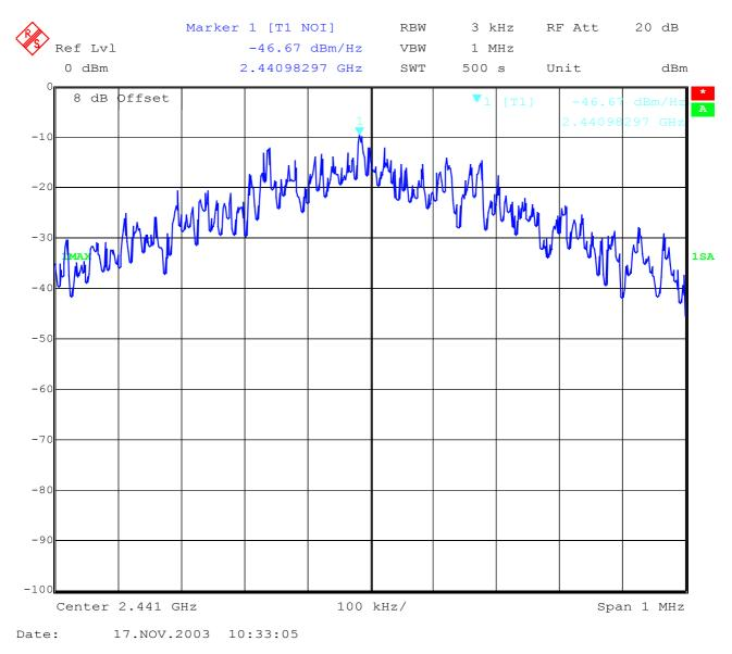
Power density : -46.67 dBm/Hz = -11.87 dBm / 3 KHz
