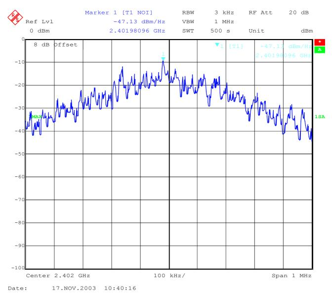
Power density : -47.13 dBm/Hz = -12.33 dBm / 3 KHz
