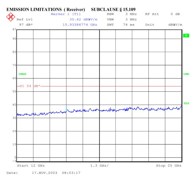
f < 1 GHz : RBW/VBW: 100 kHz Limits  $f \ge 1$ GHz : RBW/VBW: 1 MHz
