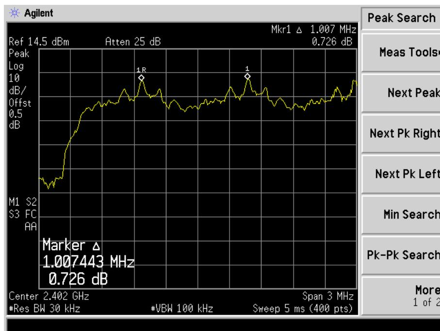
Channel Spacing (Middle CH=1MHz)
