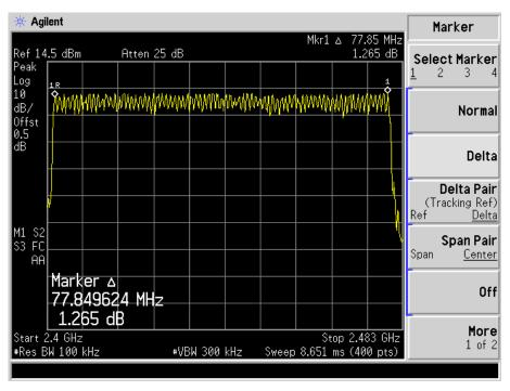
For GFSK mode Channel Spacing (Low CH=1MHz)
