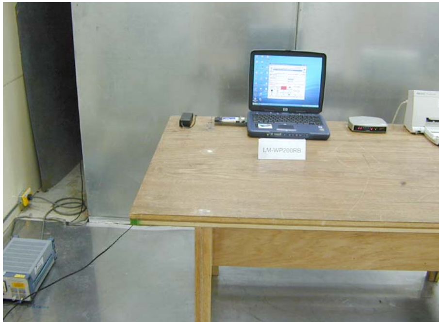
Appendix C2: Conducted Emission Test Set-up (rear)
