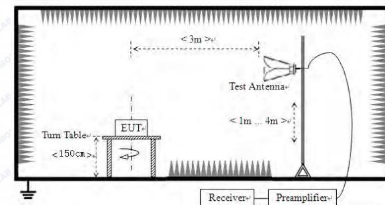
Note: For harmonic emissions test a appropriate high pass filter was inserted in the input port of AMP.
