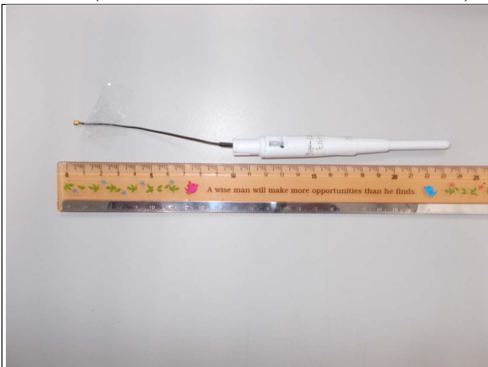
Antenna 8 (Brand: MAG.LAYERS ; Model: EDA_1313_2G4C1-A16)
