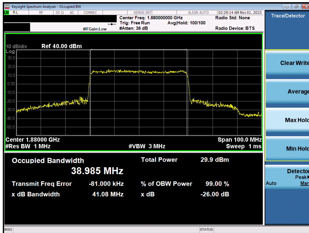
Plot 7-50. Occupied Bandwidth Plot (NR Band n2 - 40.0MHz CP-OFDM QPSK - Full RB - ANT M3)
