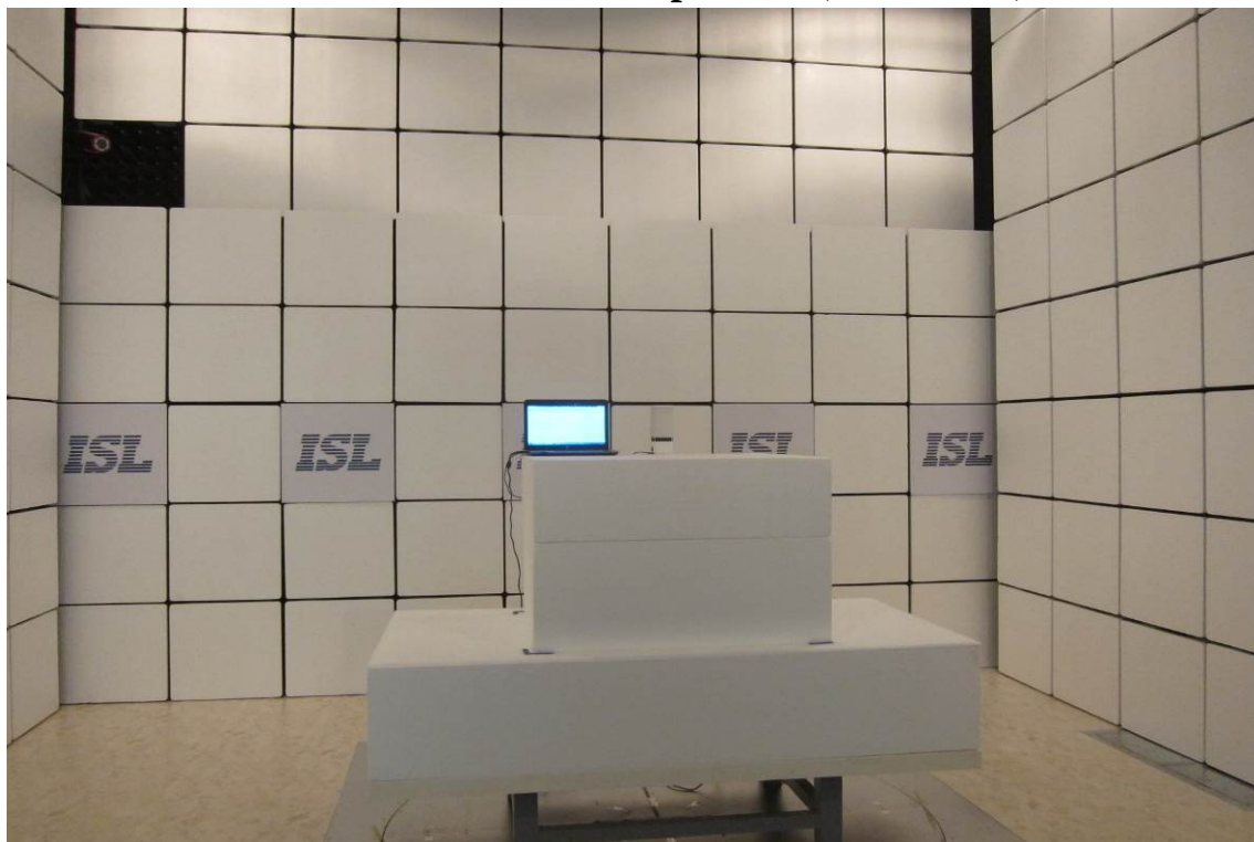
Radiated Emission Set up Photo (above 1GHz)
