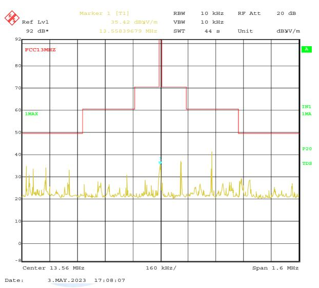
A spectrum analyser plot showing the carrier and modulation peaks within +/- 800 kHz.
