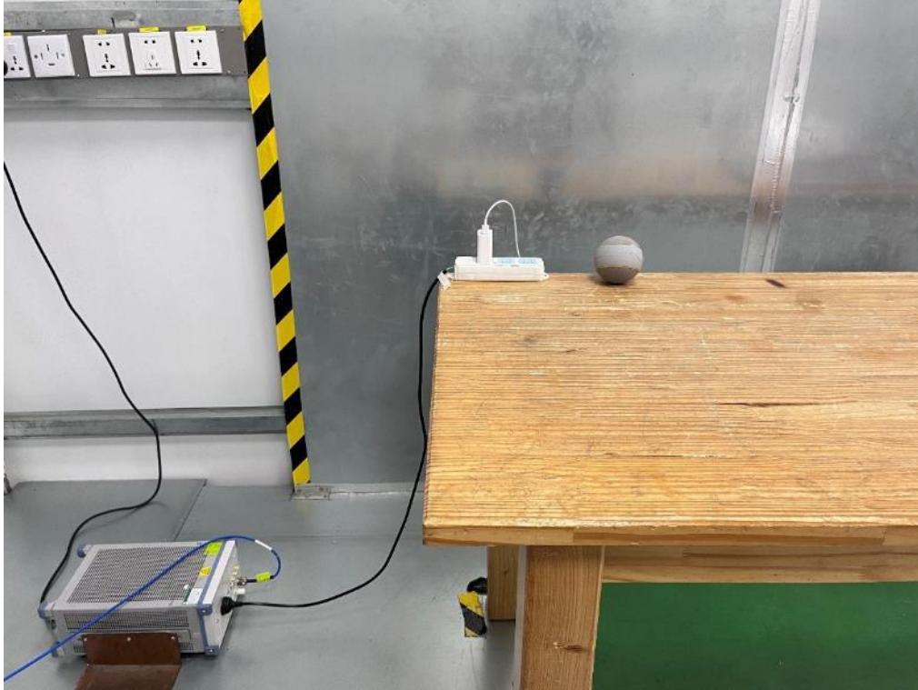
AC Power Line Conducted Emission
