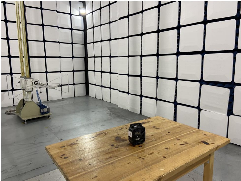
Photo of Radiation Emission Test
