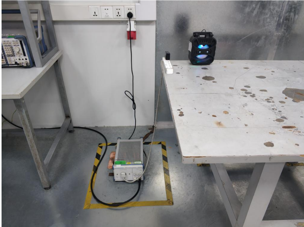
Photo of Power Line Conducted Emission Test
