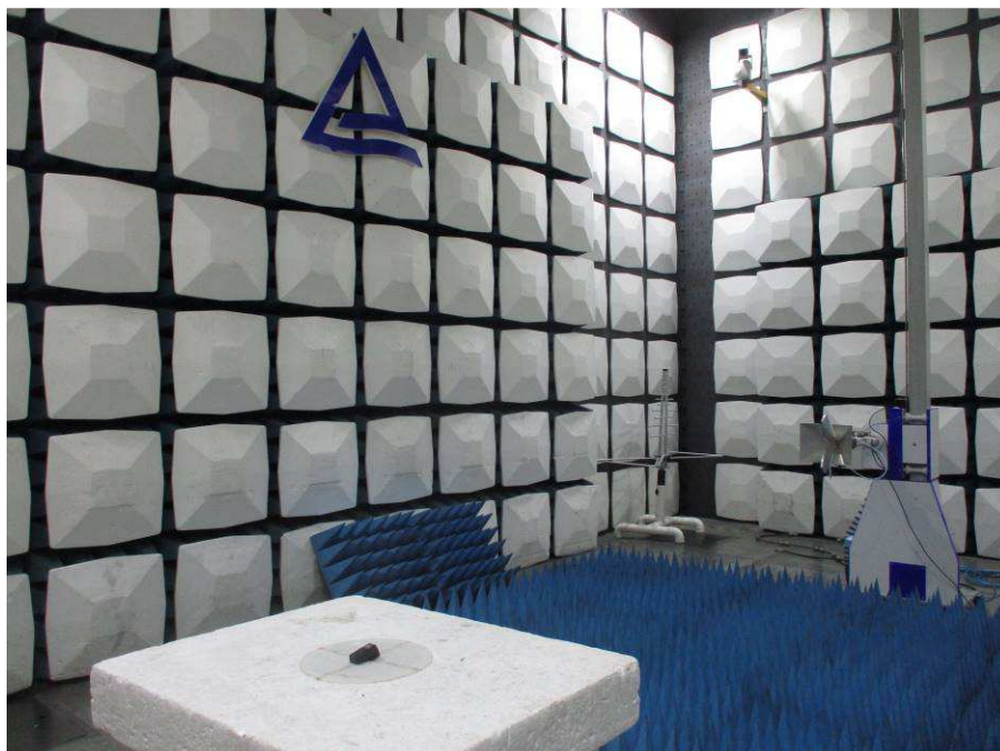
Photograph 4: Set-up photo for Radiated Emissions Above 1GHz
