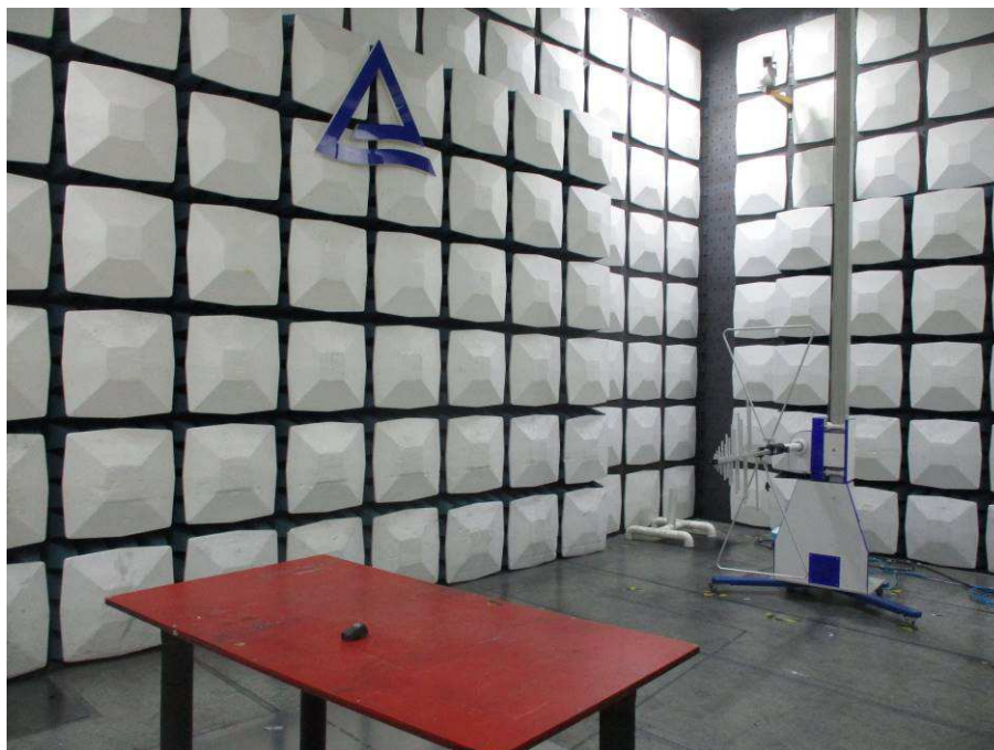
Photograph 3: Set-up photo for Radiated Emissions Below 1GHz
