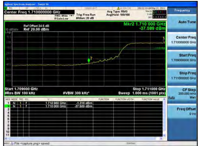
Band4 / 10MHz / High CH / QPSK / FULL RB
