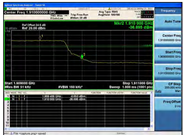
Band2 / 5MHz / High CH / QPSK / FULL RB
