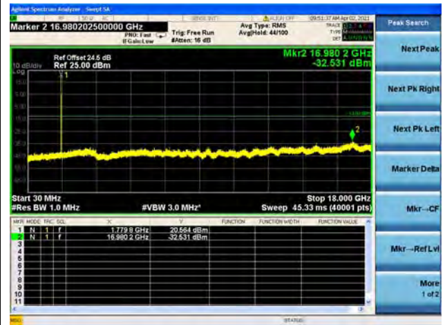
Band66 / 3MHz / Low CH / QPSK
