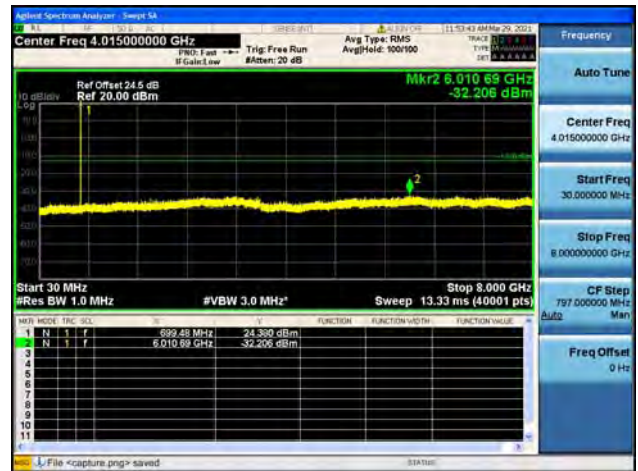
Band12 / 1.4MHz / Mid CH / QPSK
