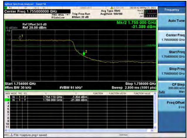
Band4 / 5MHz / Low CH / QPSK / FULL RB
