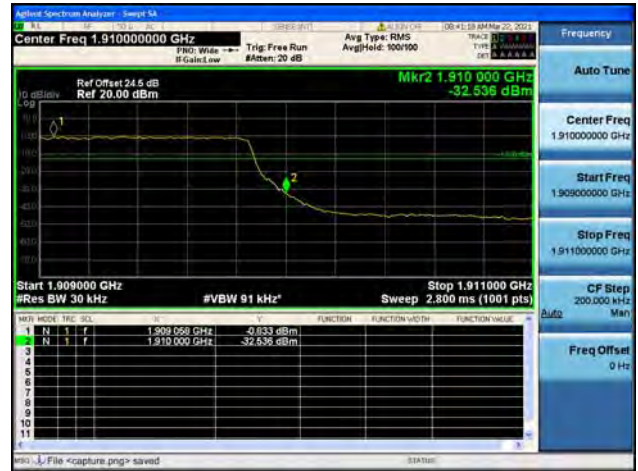
Band2 / 5MHz / Low CH / QPSK / FULL RB
