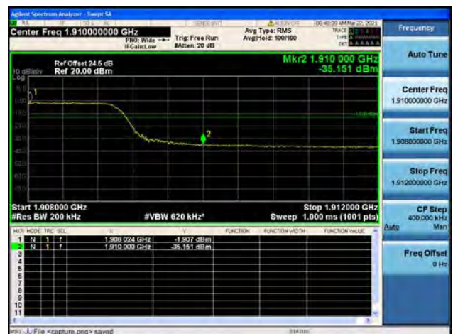
Band2 / 20MHz / High CH / QPSK / FULL RB
