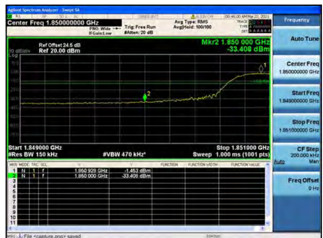
Band2 / 15MHz / Low CH / QPSK / FULL RB
