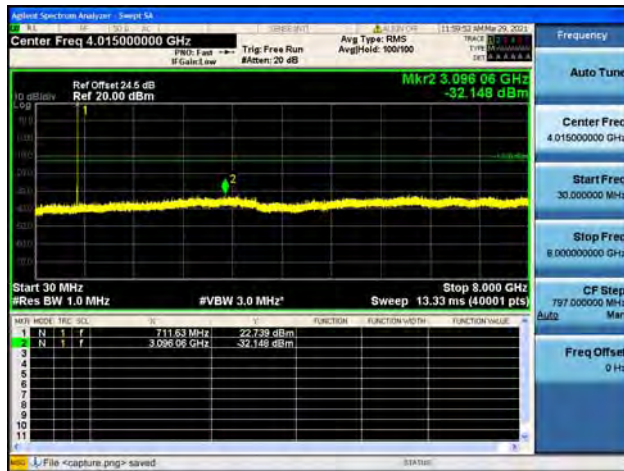
Band12 / 5MHz / High CH / 64QAM
