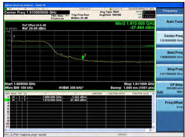
Band2 / 15MHz / Low CH / QPSK / FULL RB
