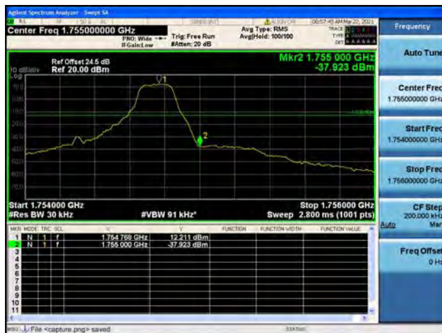
Band4 / 3MHz / Low CH / QPSK / 1 RB
