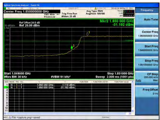
Band2 / 3MHz / Low CH / QPSK / FULL RB
