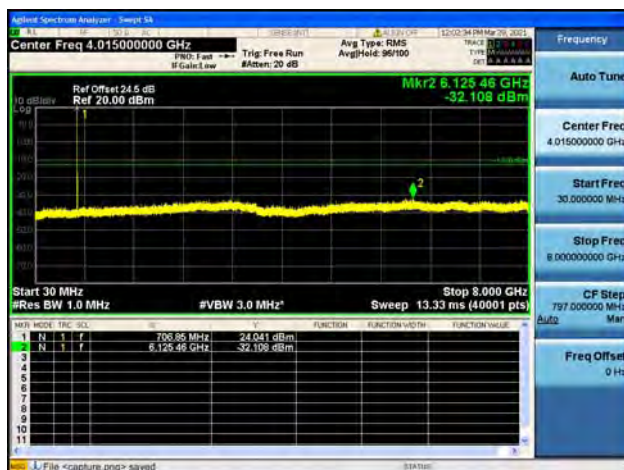
Band12 / 10MHz / High CH / 16QAM
