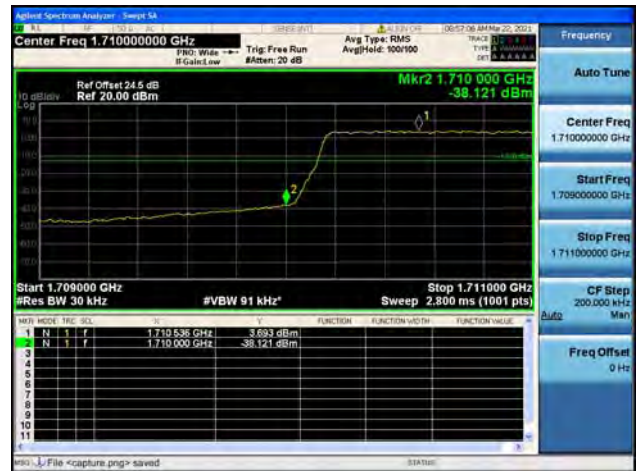
Band4 / 1.4MHz / High CH / QPSK / FULL RB
