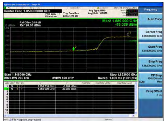
Band2 / 20MHz / High CH / QPSK / FULL RB
