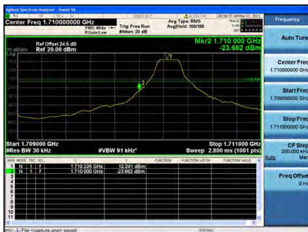
Band4 / 3MHz / Low CH / QPSK / 1 RB
