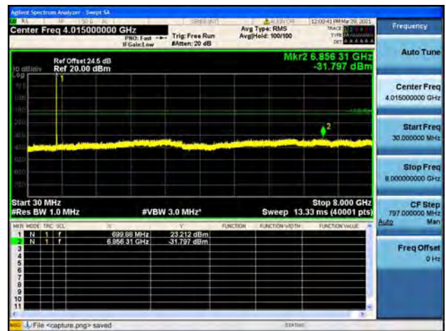
Band12 / 10MHz / Low CH / 64QAM
