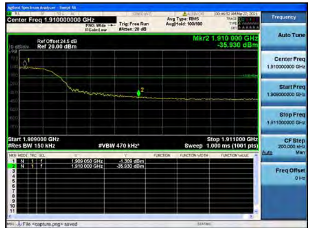
Band2 / 20MHz / Low CH / QPSK / FULL RB
