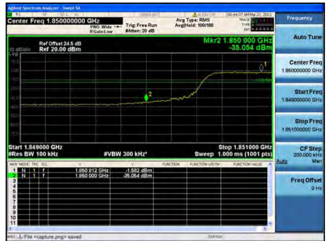
Band2 / 10MHz / High CH / QPSK / FULL RB
