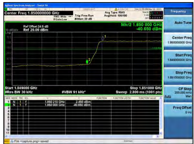
Band2 / 1.4MHz / High CH / QPSK / FULL RB
