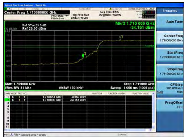
Band4 / 5MHz / High CH / QPSK / FULL RB
