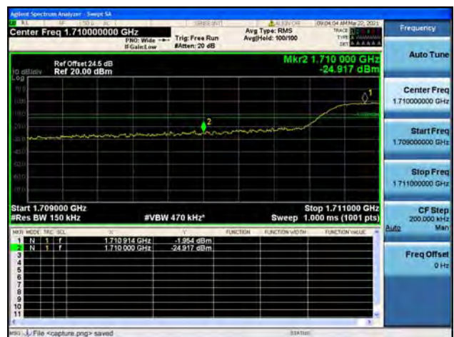
Band4 / 15MHz / Low CH / QPSK / FULL RB
