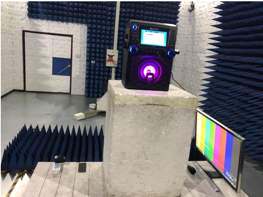
RADIATED EMISSION TEST SETUP ABOVE 1GHZ
