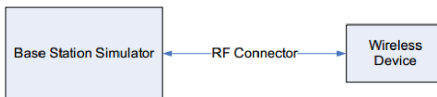
Figure 9.1 Power Measurement Setup
